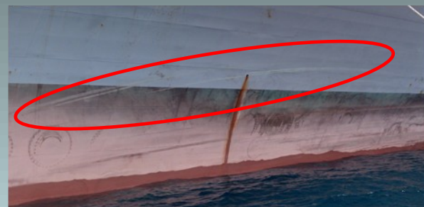
Figure 2: The scratches on the port bow of MAERSK LAUNCESTON
