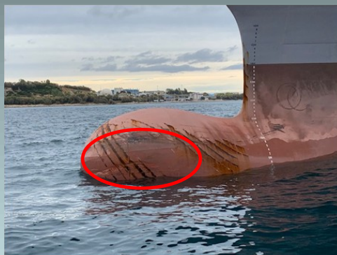
Figure 1: The abrasions in the bulbous bow of MAERSK LAUNCESTON
